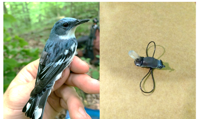
Fig. 1. Adult male Cerulean Warbler ( Setophaga cerulea ) marked with a light-level geocator (model P30Z11-7-DIP-NOT; left). Geocator (with light stalk; model W50Z11-DIP-NOT; right) and harness that goes around an individual's legs allowing the geocator to sit on the bird's synsacrum. Geolocators were manufactured by Migrate Technologies Ltd. (Cambridge, UK).
